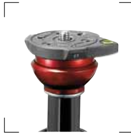
Center column with built-in 50mm half ball locked using the rotating grip located at the bottom of the center column. Tilt range: +15°/-15°.
