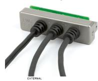
The two balanced audio outputs and the power cable are secured to the panel with rugged strain reliefs. Cables are 6 feet long and audio cables are shielded. No connectors are provided.
