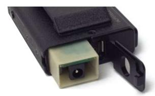
The ISO9VOLTM model is a kit including the battery eliminator and a modified battery door that fits any Lectrosonics UM type belt-pack transmitter with a hinged type door as shown here.
