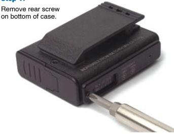
**Note:** Depending on date of manufacture, frequency adjustable models may or may not have a sliding door and bezel on this side. The screw is in the same location on both versions.
