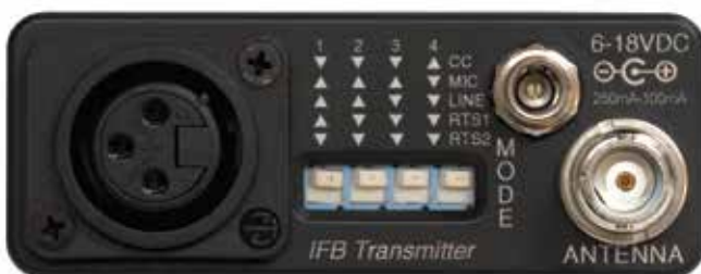
The rear panel provides the audio input and programming DIP switches for intercom and audio input type along with power and antenna input jacks.
