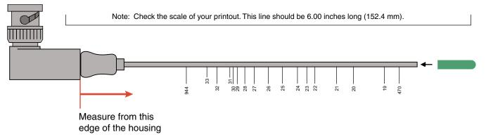
Lectrosonics A500RA UHF transmitter antennas follow the color code specifications in this chart to identify operating frequency block range. (The frequency block range is engraved on the outside housing for each individual transmitter.) If a situation exists whereby the antenna is defective and the antenna cap is missing, refer to this chart to determine the correct replacement antenna.
