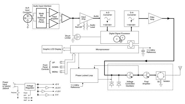
release limiter followed by a slower attack and release limiter. The dual release limiter recovers quickly from brief transients but recovers more slowly from sustained high levels, keeping audio distortion low while preserving short term dynamic changes. When the audio meter on the LCD display widens slightly as it reaches zero, limiting is indicated. When the zero changes to a letter C, severe limiting and/or clipping is indicated.
