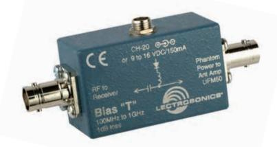
The BIAST (Bias-tee) is used to insert DC power into a coaxial cable to power a Lectrosonics remote antenna amplifier or filter/amplifier. It is positioned at the receiving end of the coaxial cable to pass DC power from an external source to the coaxial cable running to the antenna.
