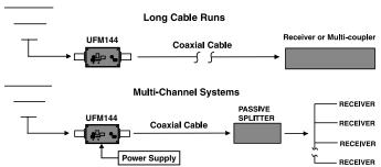
The UFM144 is placed near the antenna to apply gain ahead of long cable runs, or to compensate for splitter and cable loss in a multi-channel signal distribution system. A power supply for the UFM144 must be used since the passive splitter will not pass DC supplied by the receivers.
