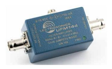
The RF amplifier is fixed at 12 dB of gain. Adjustments to the gain are made by inserting attenuators. The gain can be adjusted to +12dB, +8dB or +5dB using the 0, -4 and -7 jumpers. Remove the four screws and the bottom cover for access to the internal connections and jumpers.
