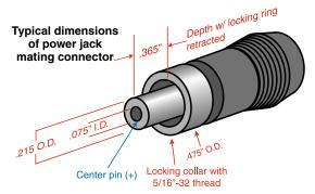
Mating split-pin on side panel jack may need to be widened slightly for a secure fit
