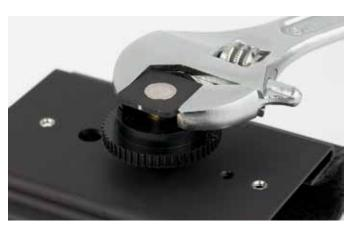
2. Use a wrench to thread the stud in about 1 - 2 turns, then rotate it to orient the receiver control panel in the desired direction.
