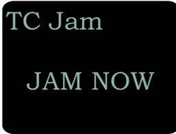
When TC Jam is selected, **JAM NOW** will blink on the LCD and the unit is ready to be synced with the timecode source. Connect the timecode source and the sync will take place automatically. When the sync is successful, a message will be
