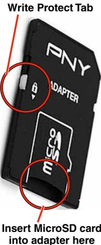
**NOTE:** The MicroSD card adapter has a write protect tab. Sliding the tab downward to the locked position prevents recording of data and protects existing data. When recording to, erasing from or formatting the MicroSD card, slide the tab upward.
