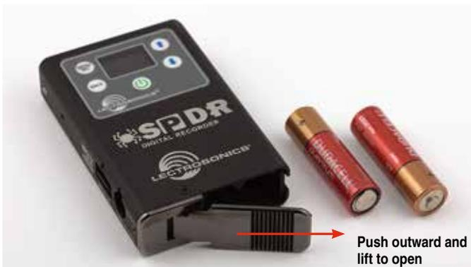
Insert the batteries according to the markings on the back side of the housing.
