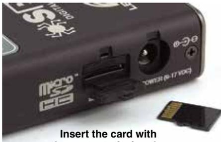
Insert the card with the contacts facing the control panel side of the recorder.
