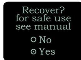
If "No" is chosen, nothing is done to the card and the SPDR will not use the card. If "Yes" is chosen", a prompt appears asking for the length of the recording to recover, specified as a number of hours and minutes. The default suggestion will be the approximate length of the most recent recording. It is always safe to recover a longer recording than was made. To specify the recovery time, use the MENU/SEL button to navigate and specify the hours and minutes fields.
