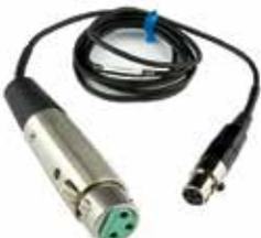
**MC41** mic level adapter cable. Female XLR to female TA5F; 37 inches long. Feeds mic level signal to pin 3 on the TA5M jack.
