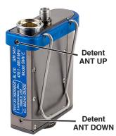
Two detents in the flat side of the housing align the belt clips. The antenna UP version is shown. Align the bracket so the set screw seats into the detent and tighten it with the hex key. Do not overtighten the set screw.
