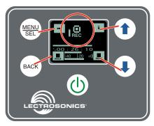
In Playback Mode, the soft buttons on the LCD change to provide the functions needed during playback. There are three variants of playback
