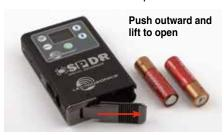
Insert the batteries according to the markings on the back side of the housing.
