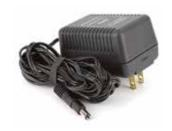
The SPDR is designed to be used with the CH12 external (or equivalent) power source. The nominal voltage to operate the unit is 12 VDC, although it will operate at voltages as low as 6 VDC and as high as 17 VDC. External power sources must be able to supply 200 mA continuously.
