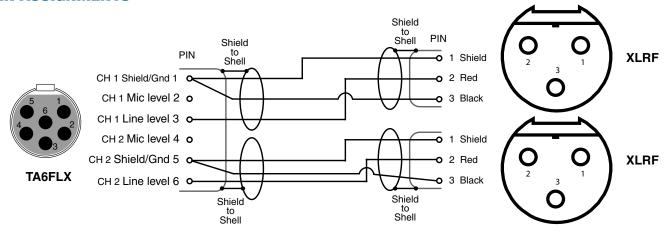
This cable is used to connect the input of the Lectrosonics Digital Camera Hop Transmitter to the analog output of a mixer or receiver. It is constructed with a TA6FLX jack, ultra flexible cable and (2) 3-pin female XLRF connectors. The connectors have soldered connections to the cable, allowing them to be serviced or replaced if the need arises.
