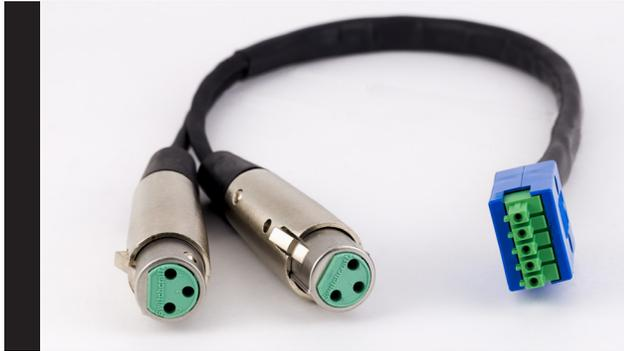
This adapter cable provides a convenient interconnection between an audio source with XLR-M output connectors and the input of a Lectrosonics device with Phoenix connectors. A common use is to connect the output of a Lectrosonics Venue 2 receiver to the DNTBOB88 breakout box to feed a Dante network. Other uses include connecting microphones to Lectrosonics processors.
