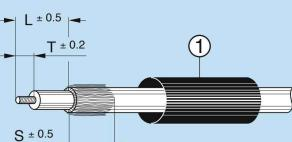
① heatshrink boot to be placed on cable if desired
