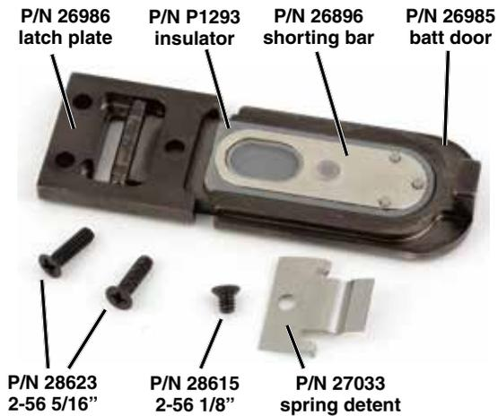
Assemble the battery door and latch plate.
