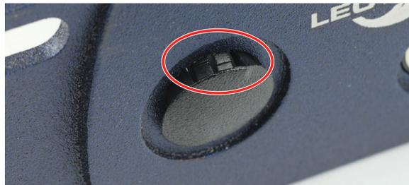
Use a small, flat blade screwdriver to press downward on the retaining tabs. Place a piece of thick paper (card stock) between the screwdriver and the panel to avoid scratching the finish, and pry outward to remove the hole plug.
