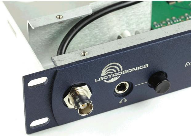
Antennas can still be connected to the rear panel by simply disconnecting the internal cable at the rear panel BNC connector.
