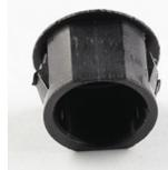
The hole plugs on the front panel have retaining tabs on two sides. In order to remove them, press down on the tabs with a flat screwdriver on the top of the plug **while pushing outward on the plug with your thumb or finger**. The plug will be partially exposed.
