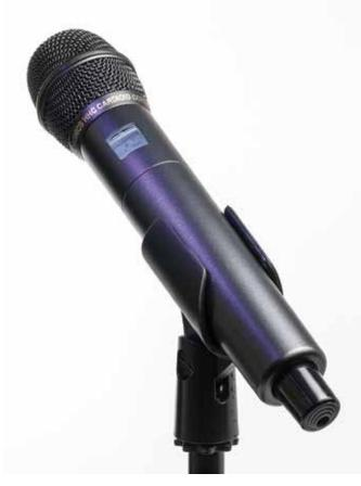
The transmitter benefits from a fourth generation design with specially developed, high efficiency digital circuitry for extended operating time on two AA batteries. The transmitter can tune across the UHF television band from 470.100 to 607.950 MHz (470.100 to 614.375 for export), with a selectable output power of 25 or 50 mW. The pure digital architecture enables AES 256-CTR encryption for applications that require high level security.
