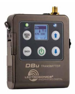
The DBu, DBu/E01 transmitter is a fourth generation design with specially developed, high efficiency digital circuitry for extended operating time on two AA batteries. The transmitter can tune in coarse or fine steps across the UHF television band from 470.100 to 607.950 MHz (DBu/E01 frequency range is 470.100 to 614.375 MHz), with a selectable output power of 25 or 50 mW. The pure digital architecture enables AES 256-CTR encryption for high level security applications.
