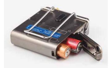
Firmware updates are made via the USB port on the side panel of the housing. The procedure is very simple using a menu item on the transmitter and a standard micro USB cable.
