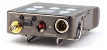
The housing is constructed of solid machined aluminum for lasting ruggedness. The exterior is finished with an ultra hard, black electroless nickel finish.
